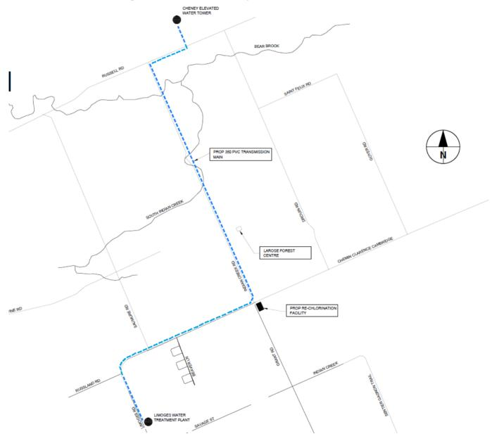
The majority of the construction will be performed using HDD methods, meaning that the pipe is horizontal directionally drilled below the surface and not open excavated. This greatly reduces the impact on all existing infrastructure and private property. All proposed work will be performed in municipal right of ways and not on private property. No service connections will be made along the alignment, as this water main is only a transmission water main.
