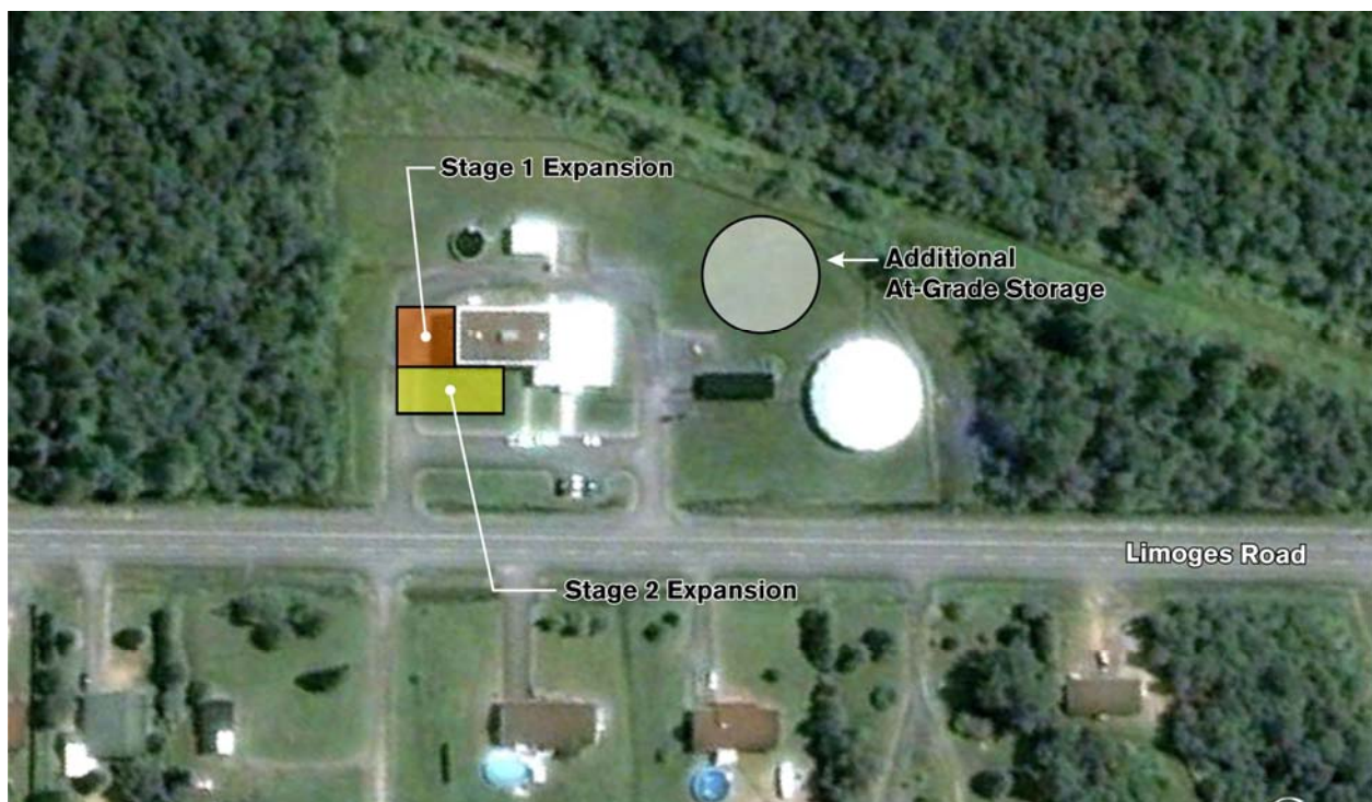
Figure 7-3: Water Treatment Plant Staging
