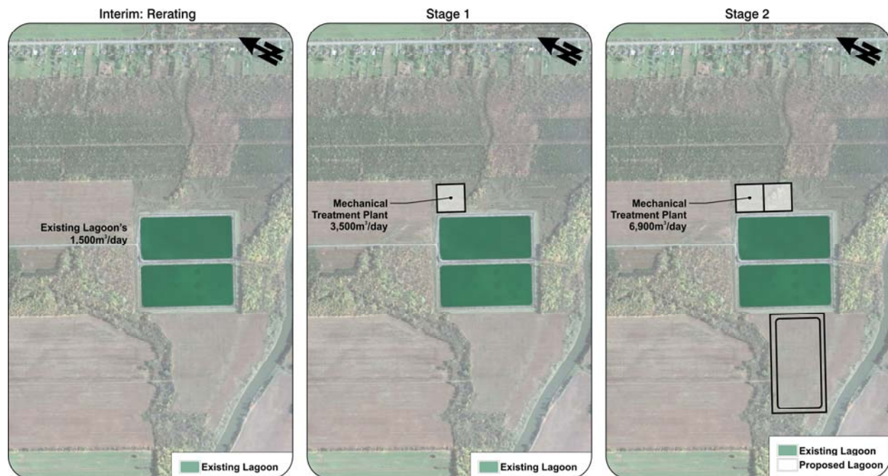
Figure 7-9: Wastewater Treatment System Staging
