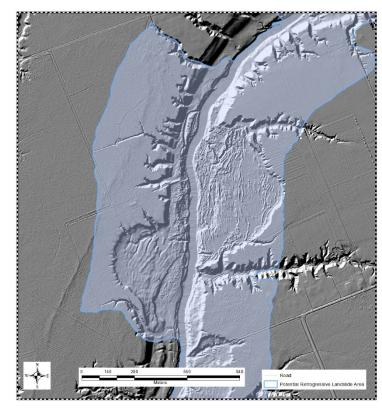
Topographical mapping (LiDAR images), 1971 Landslide scar.
