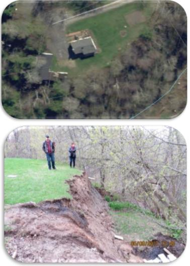
Small-Scale Landslide following unpermitted garage construction, 2017.
